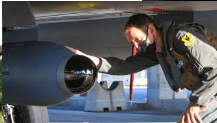
Left: SSgt Raughton. U.S. Air Force pilot inspects the IRST Pod attached to his F-15C Eagle. January 26, 2022. USAF. https://www.af.mil/News/Photos/i-photo/2002937019/mediaid/5785264/
